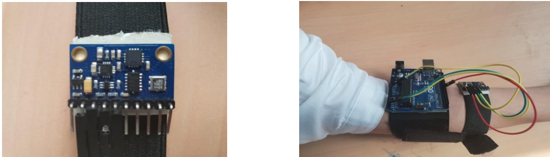
Fig 1. (a) GY-80 sensor board, (b) Placement of experimental apparatus
